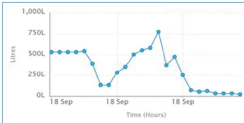
The main leakage was from a broken rubber seal attached to the evaporative air conditioners. This resulted in water running constantly through the air conditioner rather than being stored, used and disposed of as per normal operating procedure.
